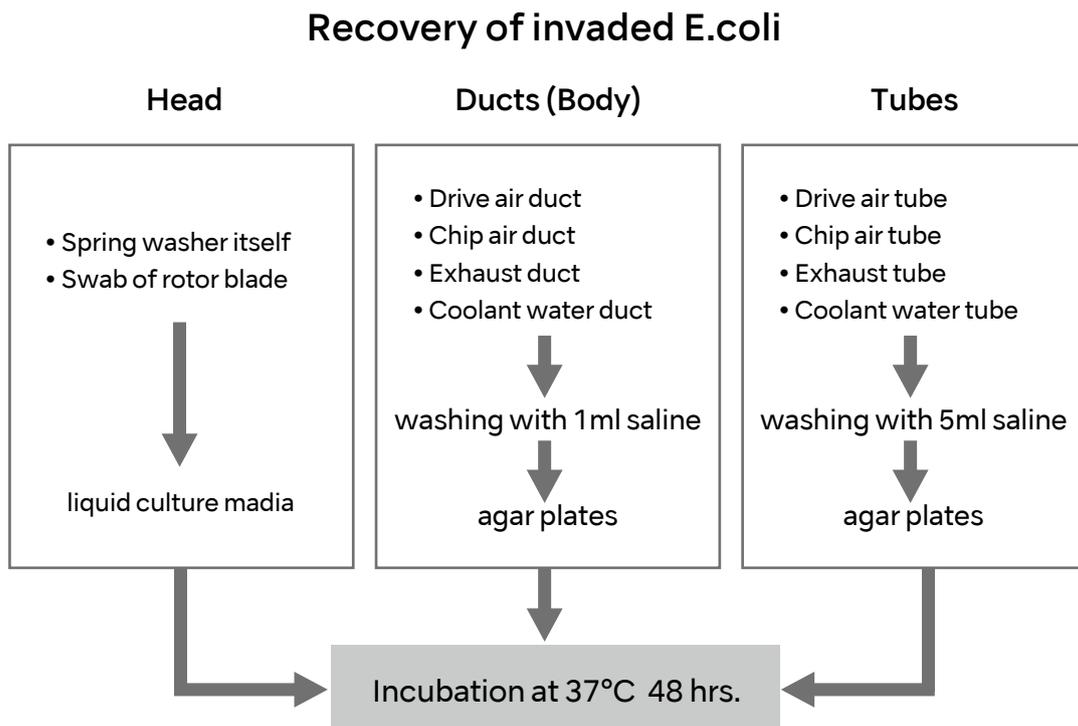
[Fig. 7] Contamination of the handpiece
